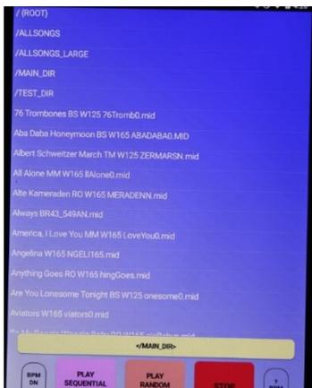
One can scroll through the list and select and play any song by tapping on it. In a similar way, one can select a new directory by tapping on it (equivalent to changing directories on a computer). Whenever a new directory is selected, a new scrolling list is automatically created with only the midi and playlist file names found in that directory. For example, if the user selects *TEST\_DIR*, a new scrolling list is created showing only the midi songs and playlists in the *TEST\_DIR* directory.
