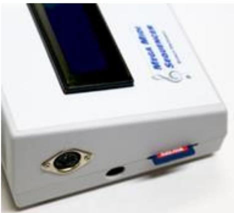
Midi I/O Connector: A standard midi compliant 5-pin female DIN connector. The digital output is midi standard compliant
