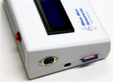
Midi I/O Connector: A standard midi compliant 5-pin female DIN connector. The digital output is midi standard compliant
